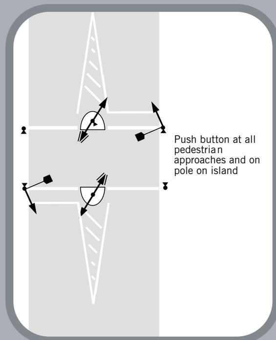
■ **Detectors** can be mounted on the traffic signal heads. These detect gaps in traffic and allow an earlier introduction of the green man crossing if there is a gap in traffic
