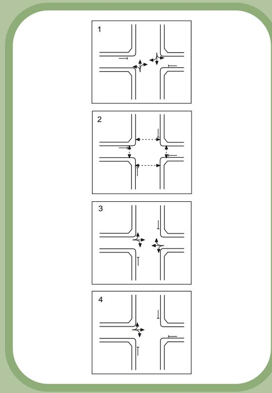
Diagram 10.10 Separately signalled right turns
