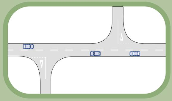
A crossroads layout can lead to a higher number of accidents than for other layouts. However it can be appropriate in low speed, low volume environments eg residential cells.
