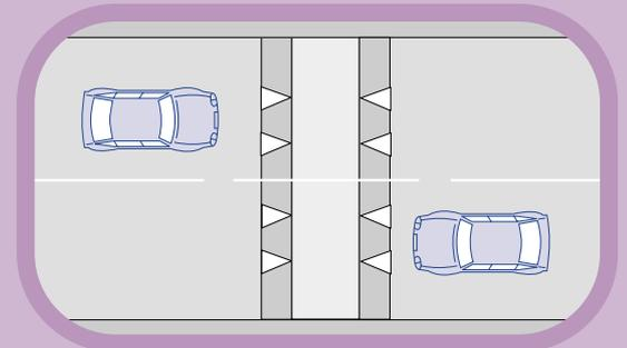
Diagram 6.34 Cross section of 75mm high flat-top ramp
