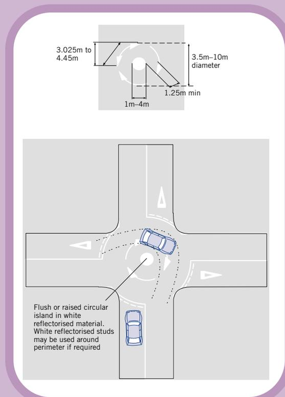
Diagram 6.13 Turning circles around mini-roundabout
