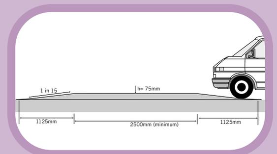
Diagram 6.35 Speed table layout at junction
