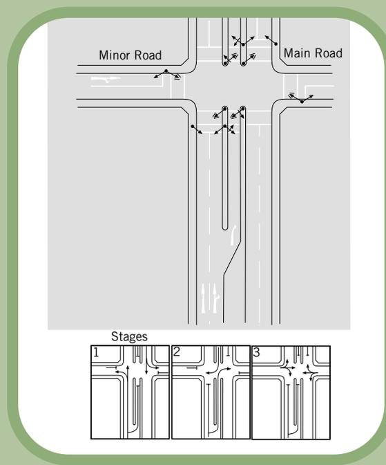
Diagram 10.10 shows an example of a separately signalled right-turn stage.
