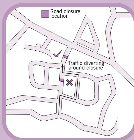
of road over which the closure is applied needs to be chosen carefully so that through traffic is diverted onto suitable alternative routes and the problem is not merely transferred onto adjacent residential roads.
