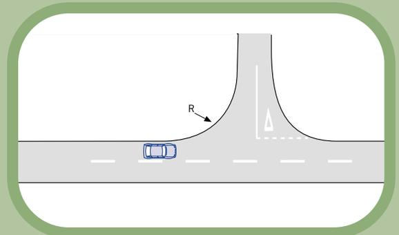
In an urban area, radii are typically 4 to 6m (with a maximum of 10m)
