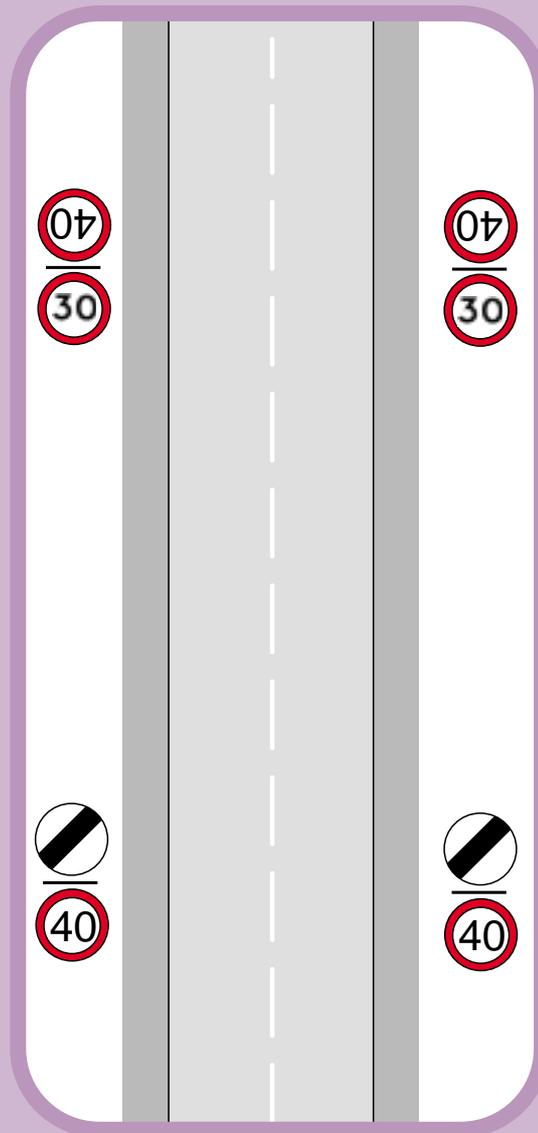
speed limit to clear a hazard such as a bend, a junction or a hump-backed bridge. The signs for the limit need to be located in a position where they can be clearly seen.
