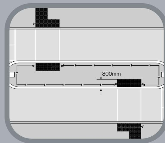
Diagram 13.7 Layout for raised entry treatment at a junction
