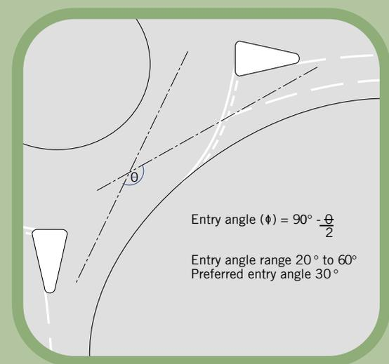
the junction and encourage high entry speeds in light traffic conditions. Where more than one lane is provided, lane widths should be between 3m and 3.5m at the entry yield line.
