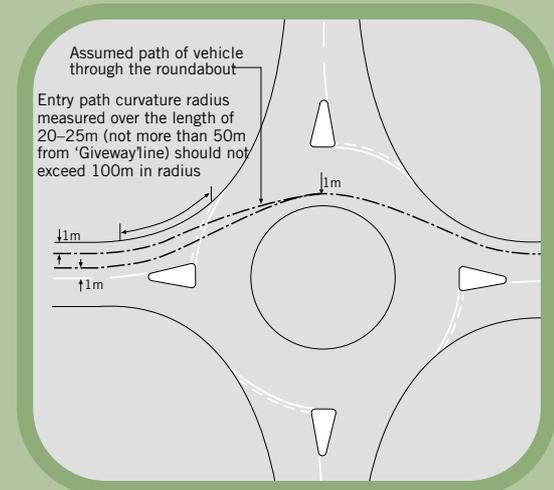
Diagram 11.7 Entry angle for a semi-rural roundabout
