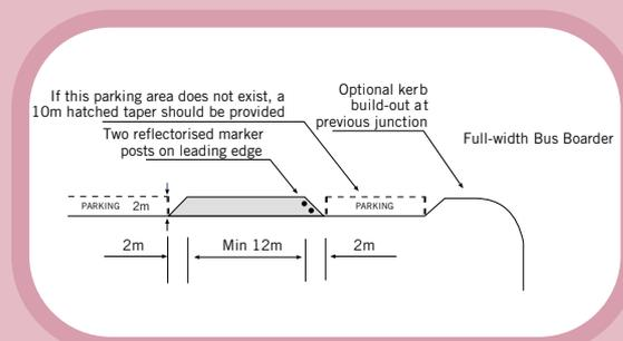
where kerbside parking space is at a premium or where it occurs with vehicles either parked at an angle or at right angles to the kerb. Bus promontories give passengers a protected route through the parked vehicles to the raised kerb. However, the disadvantage is that passenger waiting facilities cannot be provided immediately adjacent to the bus stop. They can generally be used only with single-door, front entrance buses.
