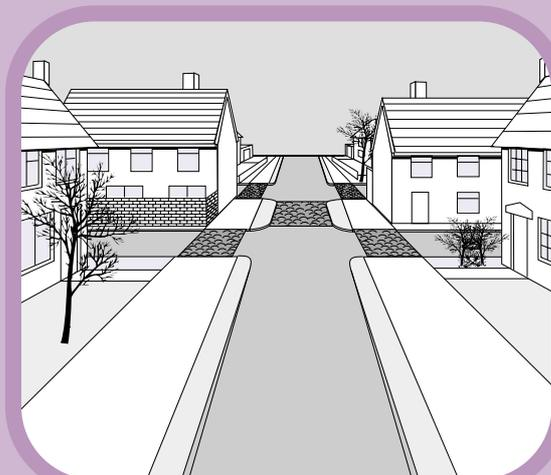
**Priority Junctions** – Drivers slow down when turning or yielding right of way at junctions. The careful positioning of priority junctions can assist in restraining speed along a length of road (see Diagram 7.8). Crossroads layouts are not recommended.
