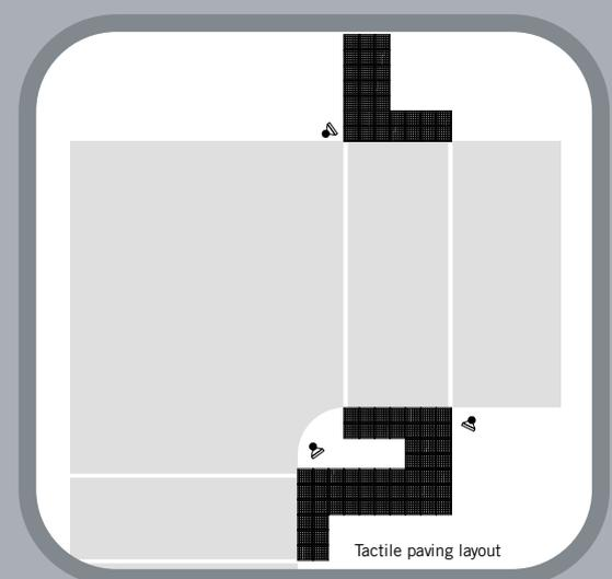
The top of the dropped kerb at the crossing should be painted white for the benefit of partially sighted pedestrians. Chamber and inspection covers should be located outside the crossing and its approaches where possible. If this is unavoidable, the tactile paving units should be laid into recessed covers to maintain the consistency of paving (see Picture 13.6). Signal controlled junctions without a pedestrian stage should be treated as uncontrolled crossings.
