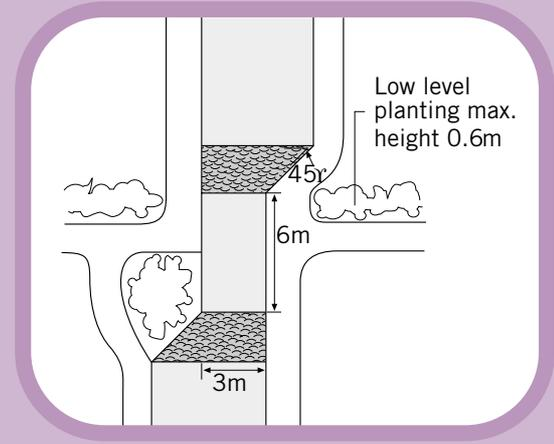
Diagram 7.4 Double speed control bend
